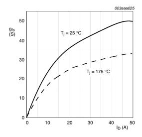
$T_j = 25$ °C and 175°C;  $V_{DS} > I_D \times R_{DSon}$
