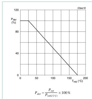
Fig 3. Normalized total power dissipation as a function of mounting base temperature
