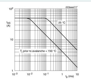
Unclamped inductive load;  $V_{DS} \le 15V$ ;  $R_{GS} = 50\Omega$ ;  $V_{GS} = 10V$
